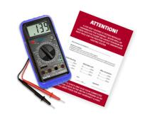
per the technical information (Point 2). Take measurements both between the resistance wires and between the resistance wire and the earth cladding.
